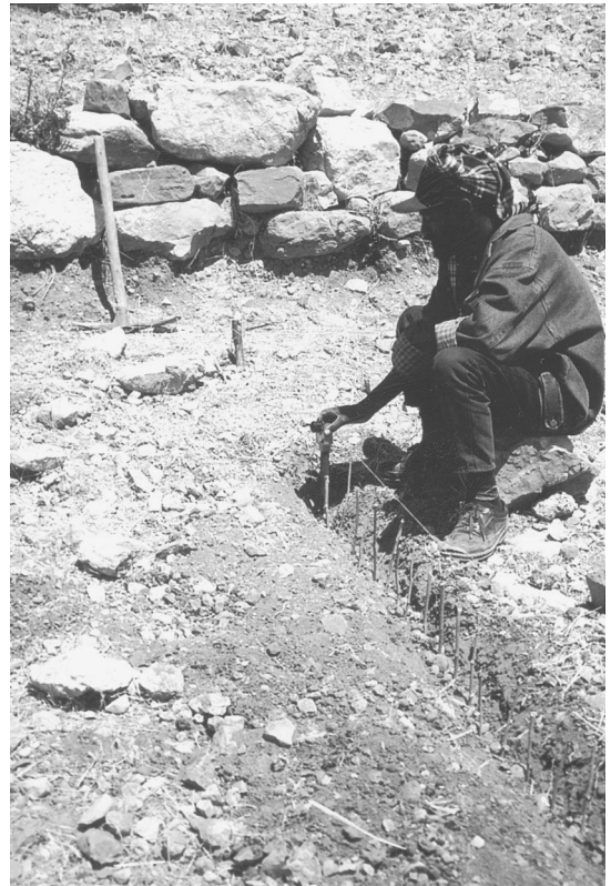
Fig. 4. Installing tracers for experiment C4. After measurement of their three-dimensional position, the tracers are covered by a thin, slightly compacted layer of soil, and another row of tracers is installed. The thin sticks serve as a guide to put the tracers in a vertical position above those of the previous rows. The exposure of the base of the stone bund (in the upper part of the photo) indicates the magnitude of soil profile truncation just downslope of it.
